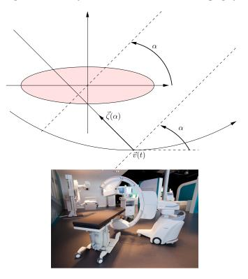
FIGURE 1 – Left : Fan Beam geometry variables  $(t, \alpha)$ . Right : C-Arm systems for the OR.
